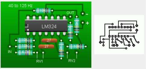
● The filter below is designed for 60Hz with adjustments for frequency and dept . Please note the voltage divider used for ground configuration .
